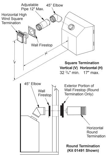
Figure 14 - Horizontal Termination Configuration for Square and Round Terminations
